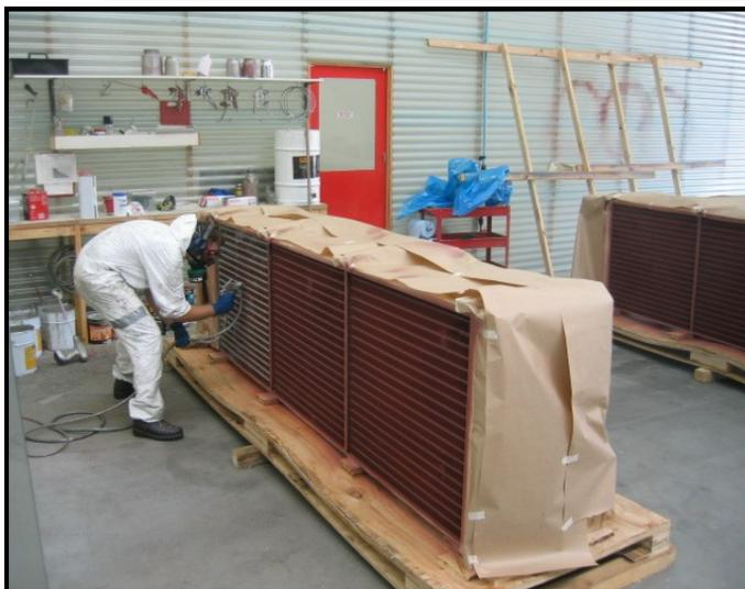
Blygold staff treating a refrigeration unit in the workshop in Queensland. Quite often these units have the same corrosion problems as the A/C chiller coils, so adequate treatment is recommended. These particular units consist of copper-copper coils in stainless steel casings.
